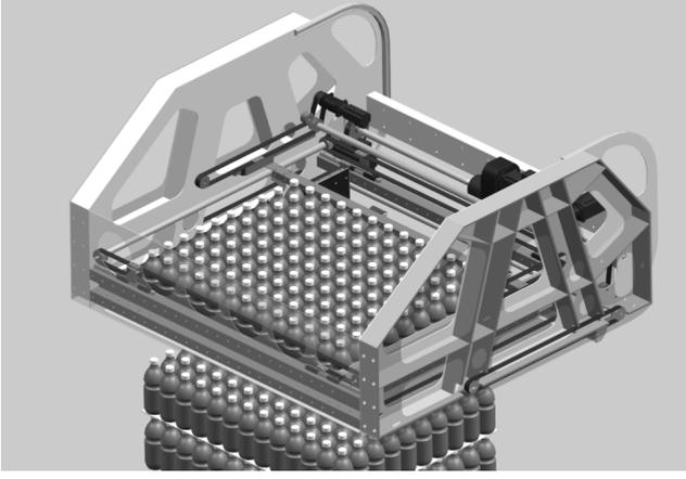
Fig. 1. Simulation of a palletizing device: a multibody problem with many frictional contacts.
