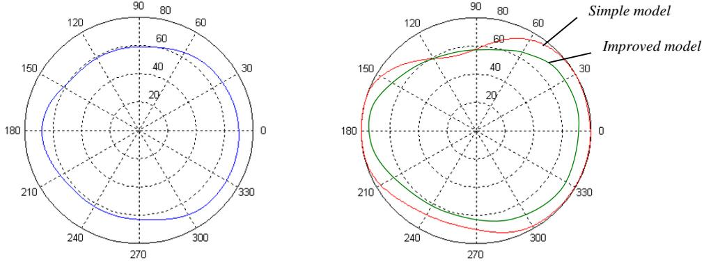
Figure 9: Experimental wear of shaft (subtracted to a circle of 80 $\mu\text{m}$ ) on the left, and numerical simulation of wear with Reye hypothesis on the right (simple and improved model).
