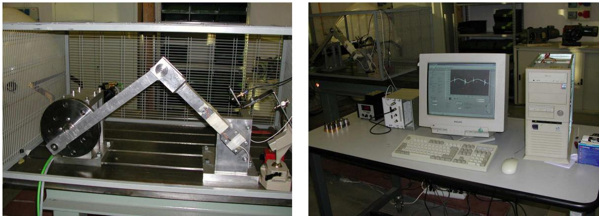
Figure 2. Instrumented four-bar mechanism and data acquisition system.
