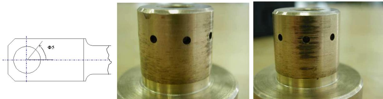
Figure 6. Surface wearing on axle, for  $\Phi_5=0^\circ$  and  $\Phi_5=90^\circ$ .
