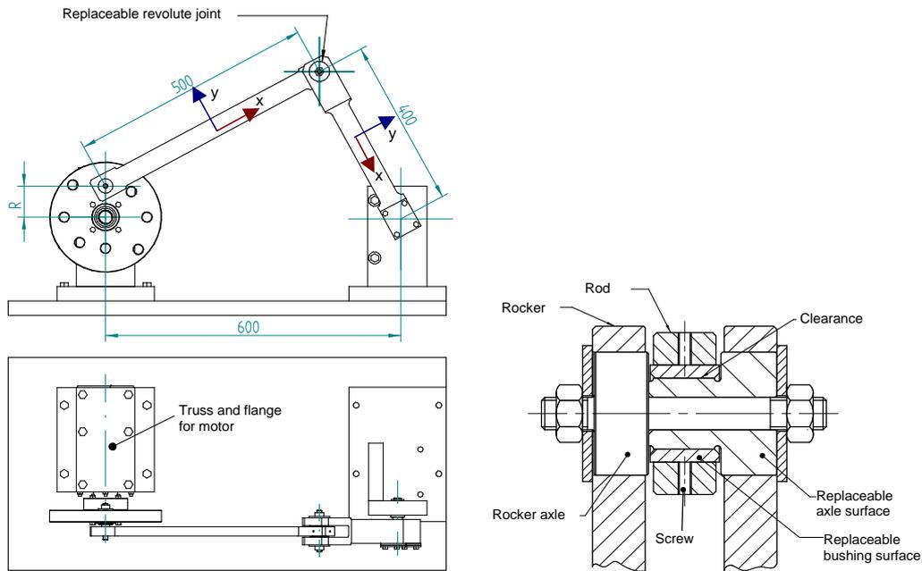
Figure 1: Design of the experimental four-bar linkage.
