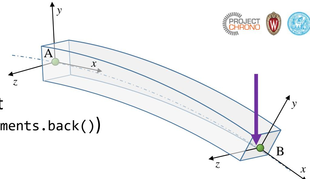
**Example: add a vertical force load to the end point of the last beam element (last element is: `beam_elements.back()`)**
